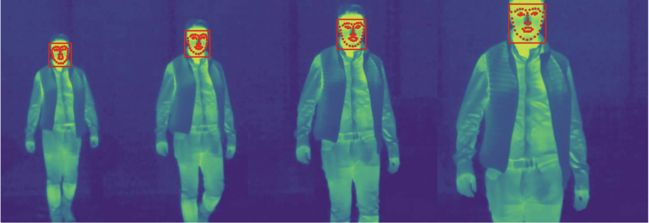
Figure 1. Monitoring system with thermal sensor. TFLD method applied on video sequence captured in the wild. A person, approximately 14m away, walks towards the camera while TFLD is tracking face and landmarks.
