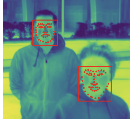
Figure 10. Examples of TFLD operating in an outdoor environment with sunny weather. Despite challenging atmospheric conditions, faces, eyes, eyebrows, nose, mouth and jawline key points are successfully located by our model. (image from TFW [9] dataset).
