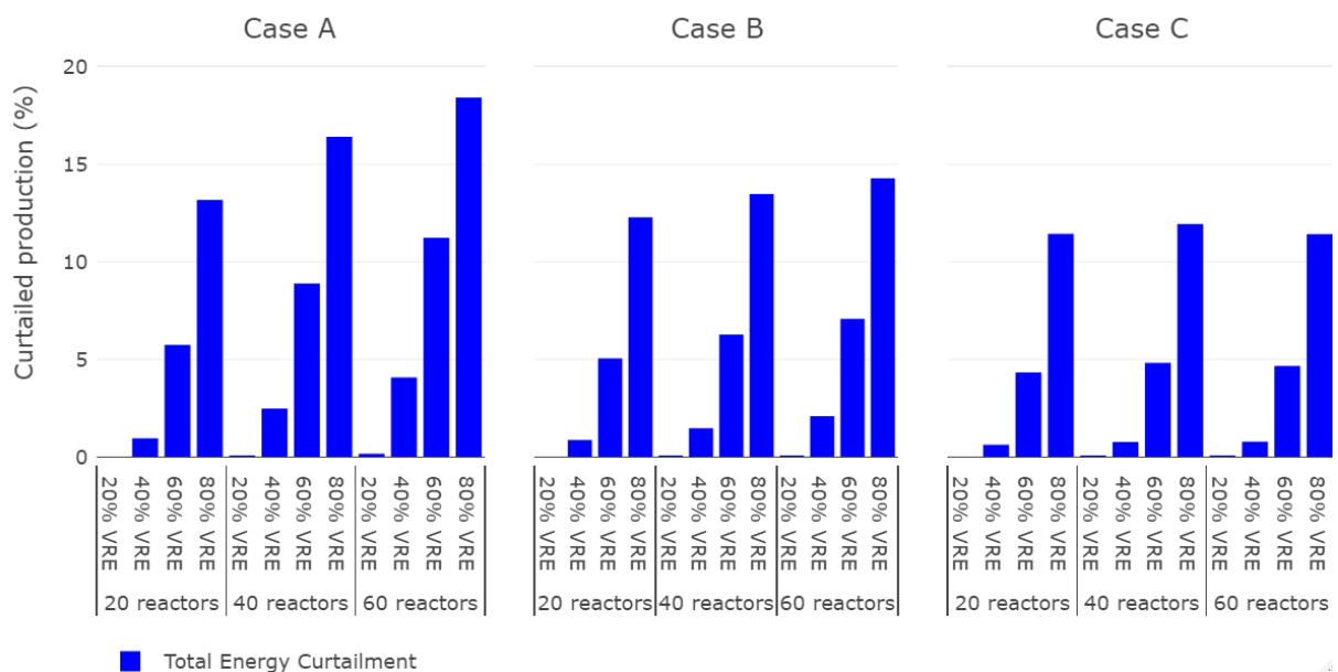
Fig. 8. Curtailed energy share for each VRE, nuclear, and nuclear flexibility assumption case (see Appendix 2 – Table A2.3).
