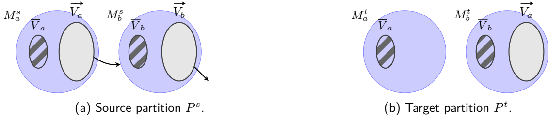
Figure 3: Illustrative example for Property 3a, where vertices in \vec{V}_a (resp. \vec{V}_b ) move from their source module M_a^s (resp. M_b^s ) (Fig. 3a) into target module M_b^t (resp. M_c^t , which is purposely not shown) (Fig. 3b). \bar{V}_a and \bar{V}_b represent the non-moving vertices.
