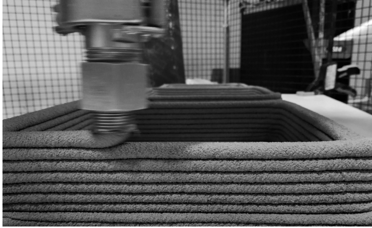
Figure 1: Concrete sample obtained by layer-wise extrusion. Geometrical heterogeneity (layering) is clearly visible, with H = 6\text{mm} , B = 20\text{mm} (Photo: Leo Demont).
