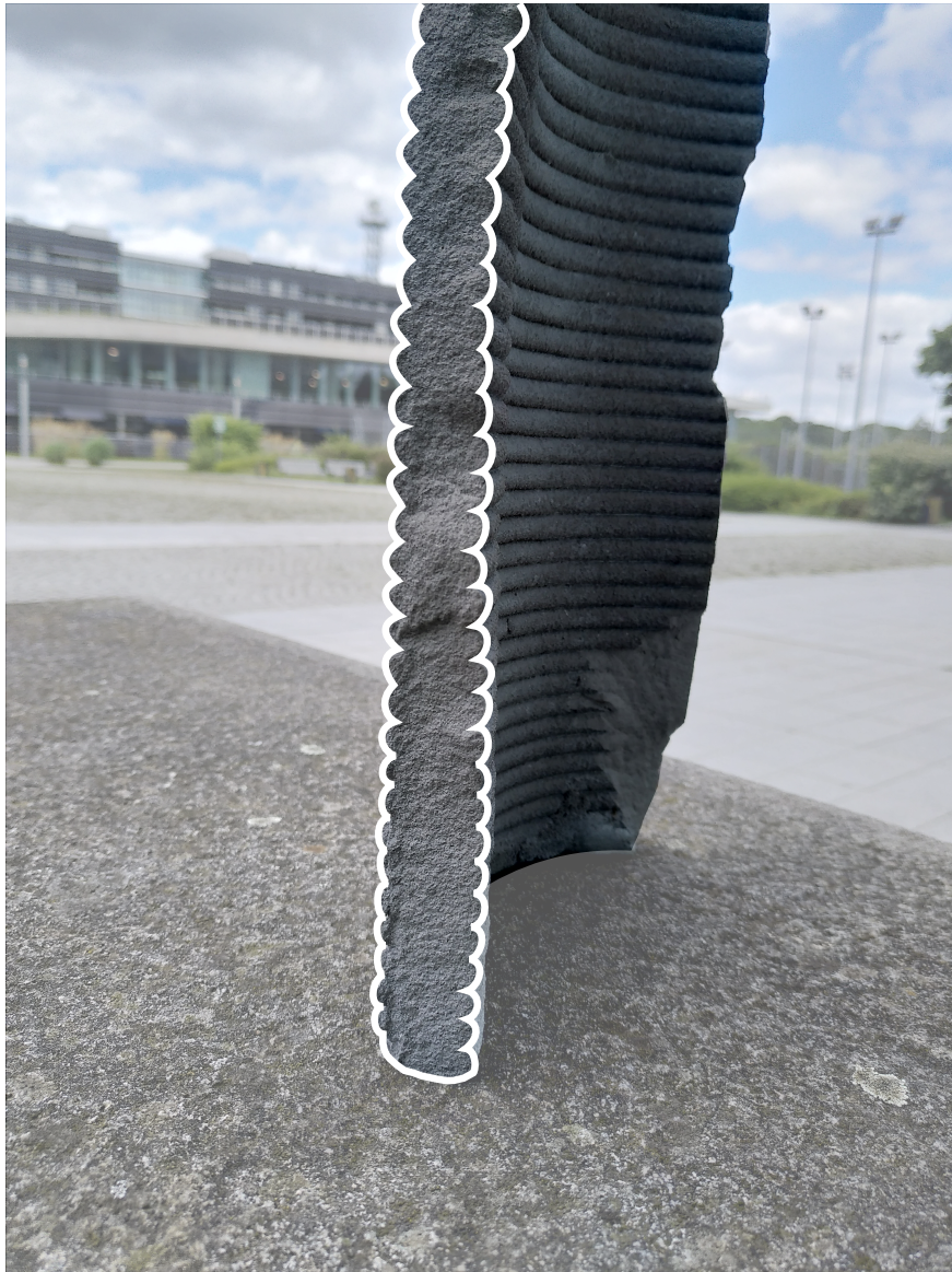
Figure 2: A crushed sample of 3d printed concrete exhibiting the oblong lace geometry (contour highlighted by the authors)
