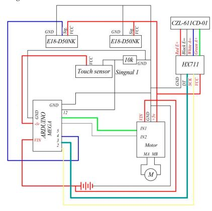
Figure 11. Connection scheme of the sensors and motor.
