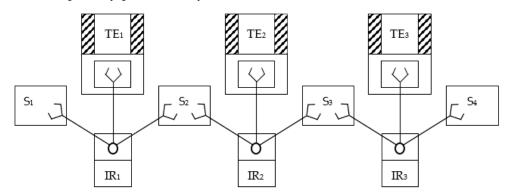
Figure 1. Scheme of a single-stream robotic cold stamping technological line.
