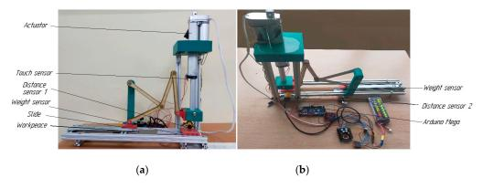
Figure 9. Prototype of the PM with two sliders: (a) the first position (b) the second position.
