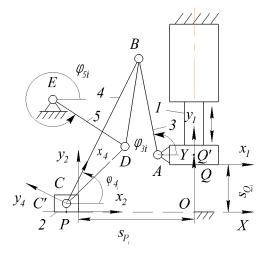
Figure 6. Intermediate position of the PM with two sliders.
