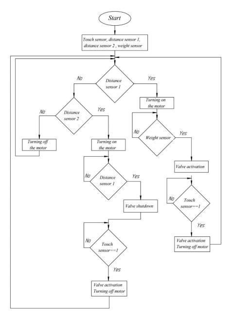
Figure 10. Block scheme of the PM with two sliders work.
