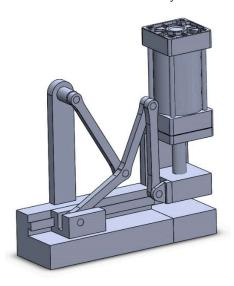
Figure 7. 3D CAD model of the PM with two sliders.
