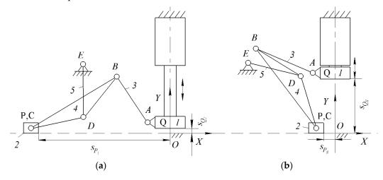
**Figure 4.** (a) lower extreme and (b) upper extreme positions of the slider Q.
