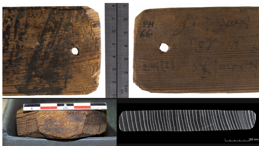
FIGURE 4 Mummy labels of different quality from the BNU collection in Strasbourg were used to acquire dendrochronological measurements. Top left: Growth rings on mummy label H087 cannot be measured easily due to tool marks and surface coating. Top right: Mummy label H066 has a clean surface and perfectly readable rings. Bottom left: growth rings on label H059 are only partly visible as a result of the cutting method applied and tool marks, the central part is illegible. Bottom right: Growth rings on the transverse plane of mummy label H043 as seen on a x-ray tomography image with perfectly legible rings
