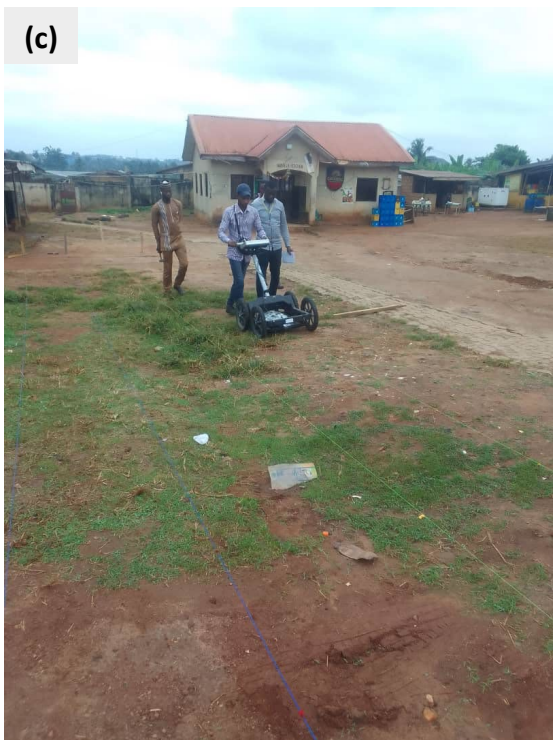
Plate 2: Photographs of Ground Penetrating Radar (GPR) survey at the Ita Yemoo site (a) setting-up of the radar (b &c) data acquisition in progress and (d) geometry and field parameters recording at the termination of a traverse measurement
