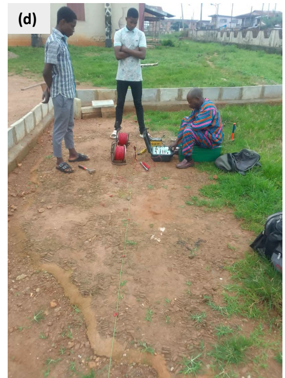
Plate 3: Photographs of resistivity survey at the Ita Yemoo site (a-c) data acquisition in progress at the main site and (d) at the outcropped potsherd pavement site
