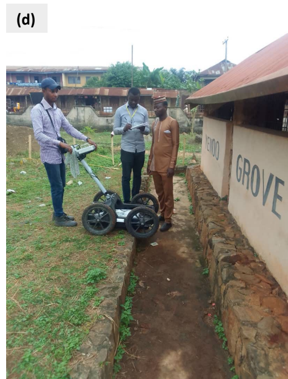
Plate 2: Photographs of Ground Penetrating Radar (GPR) survey at the Ita Yemoo site (a) setting-up of the radar (b &c) data acquisition in progress and (d) geometry and field parameters recording at the termination of a traverse measurement
