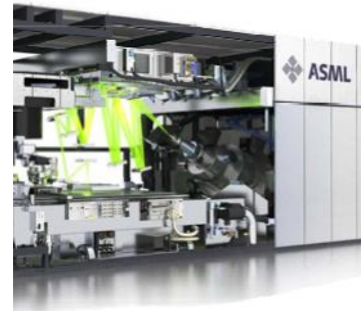
Photolithography @ 13.5 nm, 6.x nm
