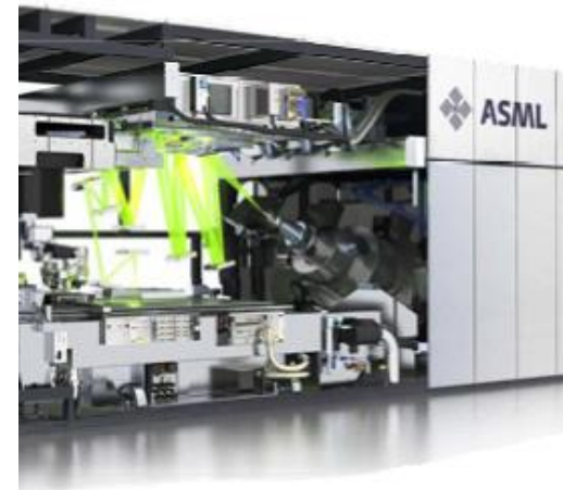
Photolithography @ 13.5 nm, 6.x nm
