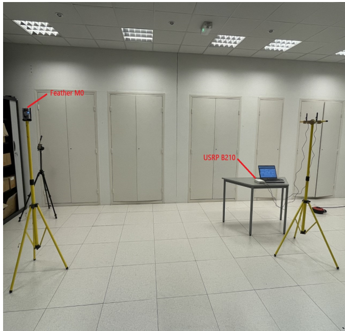
Fig. 3. The complete installation setup. Both Feather M0 and USRP B210 are fixed on the tripod.
