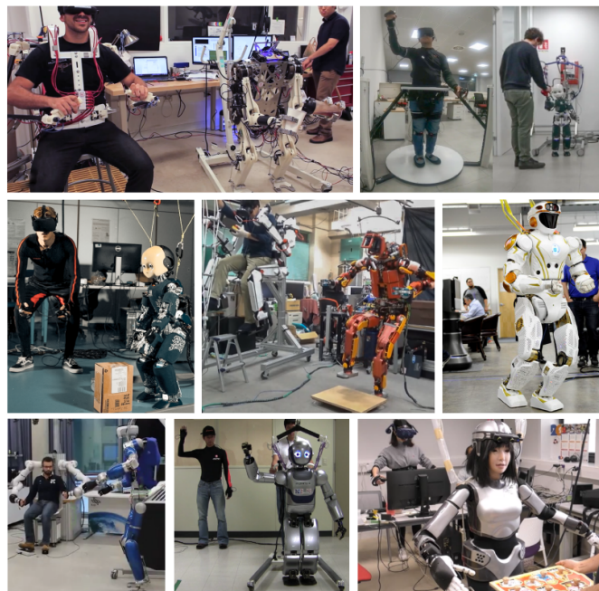
Fig. 1: Examples of humanoid robot teleoperation; from top left to bottom right corner: [1], [2], [3], [4], [5], [6], [7], [8].
