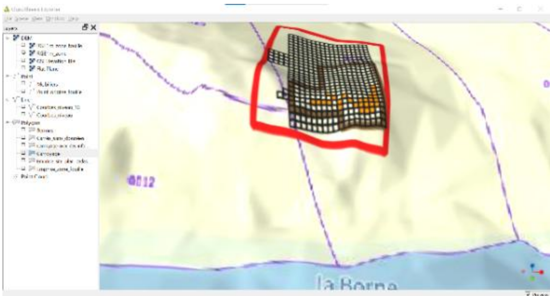
Fig. 15: 3D display in QGIS (Qgistothreejs extension) of the present topography of the site on the basis of the data from the IGN RGE ALTI 1m.
