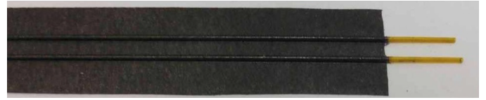
Figure 6: First prototype of the cold plate. The figure only shows one end. One coolant tube (golden) is connected to the cold plate (black) and turns 180^\circ on the other end (not shown) so that the coolant flows both directions and thus leaves on the same side it starts.
