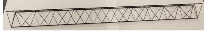
Figure 5: Prototype of the layer 5 truss, which is the longest truss. It is made from thin carbon fibre structures and evolved from the ALIC ITS2 space frame concept.
