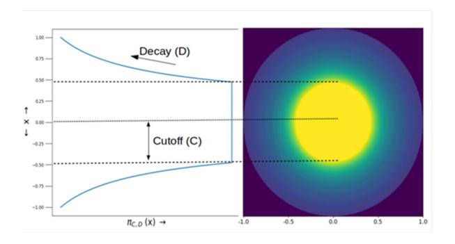
Figure 1: Target density function for SPARKLING and its parameters
