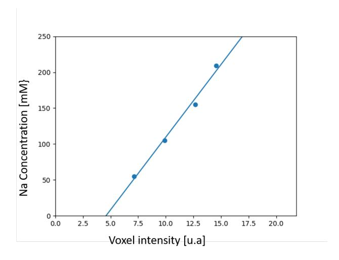
Figure S1: Example of a 4-point calibration curve for one of the *in vitro* undersampled SPARKLING (AF=128) acquisition.
