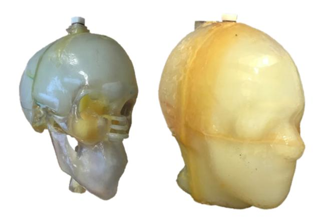
Figure 3: Anthropomorphic human head phantom. The inner and outer compartments were filled respectively with a 40 and 100 mmol/L NaCl solution. Courtesy of Thadee Delaree
