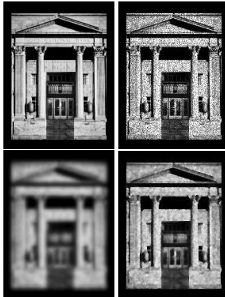
Figure 3: Examples of two dimensional diffusion filtering. The original image is on the top left and Gaussian noise was added to this to obtain the image on the top right. The two images at the bottom show the results of the diffusion filtering. The image on the left was obtained after an isotropic homogeneous diffusion corresponding to a convolution by a constant Gaussian kernel. The image on the right is the result of the inhomogeneous diffusion. The results were obtained numerically using the technique explained at the end of the report.
