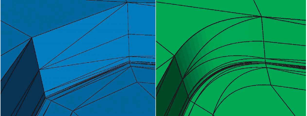
Fig. 13. Mesh around a portion of an isolated singular edges before (left) and after (right) curving.
