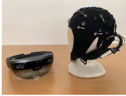
Fig. 5. Illustration of the apparatus used in the developed prototype. (Left) A Microsoft HoloLens AR headset and (Right) an mbt Smarting EEG headset.
