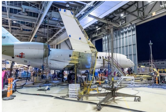
Figure 1: Falcon 6X GVT set-up
