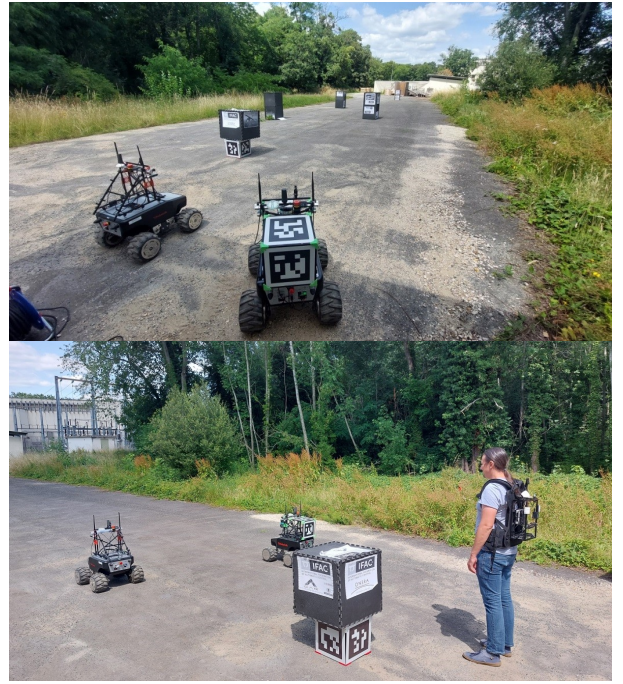
Fig. 4. Field experiments. Top: View of testing area with UGVs and obstacles. Bottom: UGVs and operator equipped with portable localization kit.
