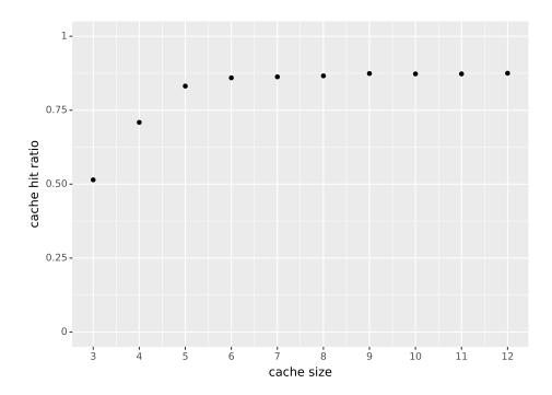
**Figure 7:** Cache hit ratio for different cache sizes on each runner. In total 128 particles run on 32 runners. The first and last assimilation cycles were disregarded to remove warm up effects and not fully recorded cycles.
