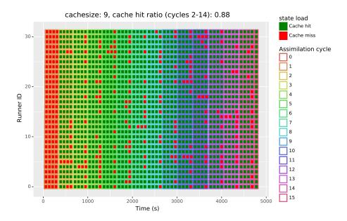
**Figure 8:** Gantt chart of particle propagations executed by the 32 runners over 15 assimilation cycles. Tasks are green if the associated parent particle state was already present in the runner cache and did not require a load from the PFS (red otherwise). For more than 97% of the cache misses (red), particle prefetching (Figure 4) is effective to load it from storage with enough anticipation not to delay its propagation.
