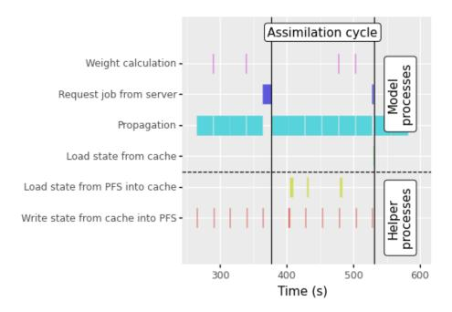
Figure 9: Trace detailing the activity of a runner over the course of an assimilation cycle. Helper processes enable to keep model processes busy with particle propagation, except at the end of assimilation cycles when they wait for the server to finish particle resampling (dark blue). Some activities are so thin that they are not visible here (state copies from cache to model).
