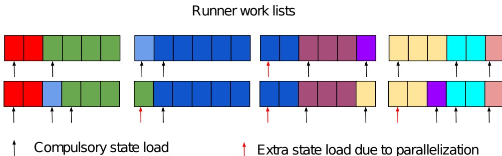
Figure 5: Two possible schedules of 24 propagation tasks of equal duration on 4 runners. All particles propagated from the same parent particle state have the same color (9 parents here). The top schedule is optimal with 9 compulsory loads (one per parent), and one for the dark blue parent that cannot fit in one runner. The bottom schedule, with 2 more state loads, is a possible one that our on-line scheduling algorithm can produce. This is not optimal but still below the general Q + R - 1 bound as the algorithm ensures that no more than R - 1 "color cuts" occur and avoids the same runner loads more than once a given parent particle state.
