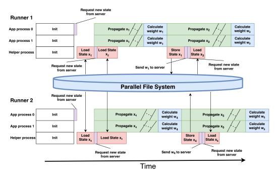
**Figure 4:** Schematic Gantt diagram showing the activity of two runners (initialization followed by two assimilation cycles). Focus on how the helper process asynchronous loads and stores enable to shadow parallel file system access. Propagation and calculation work (filled green and blue) overlap administrative work for state requests and file system loads and stores (filled violet and red)
