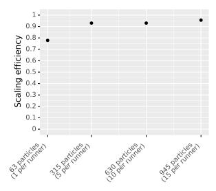
**Figure 15:** Scaling efficiency using different numbers of particles with 63 runners. One runner sets the reference case.
