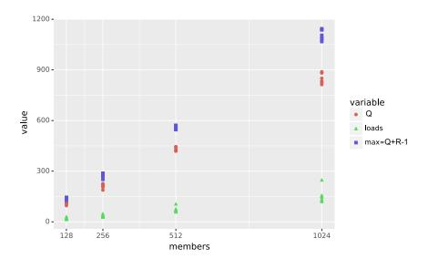
**Figure 11:** Number of parent particles Q, particles loads from the PFS to the cache, and Q + R - 1 upper bound from Equation 14 for different ensemble sizes, a cache size of 9 particles with 4 particles per runner.
