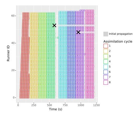
**Figure 14:** Gantt chart of particle propagations executed by the 63 runners over 8 assimilation cycles. After runners #48 and #53 crashed (black cross), two new ones restarted (top 2 runners #63 and #64).
