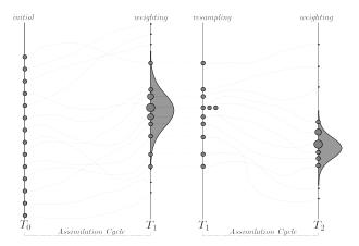
Figure 1: Initially particles are uniformly sampled. They are propagated to  $T_1$  where they are weighted taking into account observation data. Resampling leads to discarding some particles with low weights (top and bottom), while others with high weights become parents of several ones (three here). (Inspired by [38], Figure 2)
