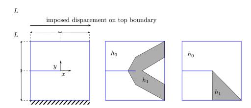
Figure 7: From left to right: shear test geometry and boundary conditions definition, mesh parameter for the symmetric case and the asymmetric case
