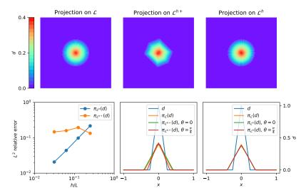
Figure B.12: Convergence of the discrete lip projection. Top, from left to right:  $\pi_{\mathcal{L}}(d)$  interpolated on the mesh,  $\pi_{\mathcal{L}^{h+}}(d)$  and  $\pi_{\mathcal{L}^{h+}}(d)$ . Bottom: from left to right, convergence analysis, cut of  $\pi_{\mathcal{L}^{h+}}(d)$  and  $\pi_{\mathcal{L}^{h}}(d)$  along the horizontal line  $(\theta = 0)$  and the diagonal  $(\theta = \frac{\pi}{4})$ , compared to d and  $\pi_{\mathcal{L}}(d)$ .
