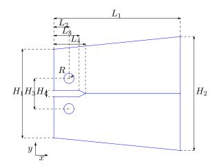
Figure 5: TDCB geometry definition.
