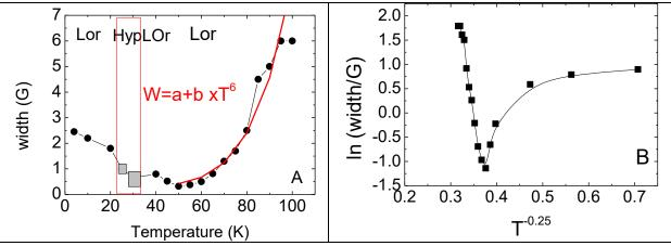
**Figure 10**: (**A**) EPR linewidth of the H shallow donor in ZnO as a function of temperature, black squares experiment, red line simulation with a power law dependence for T>50K, (**B**) tentative Mott plot of the linewidth: ln(width) vs T<sup>-0.25</sup>, experiment (black squares), the lines are only guides for the eye
