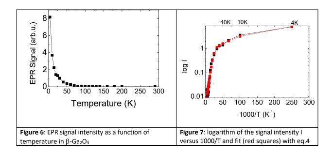
Where  $E_i$  is the thermal activation energy of process i with prefactor  $K_i$ . As shown in fig.7 the experimental data can be well fitted with two activation energies:
