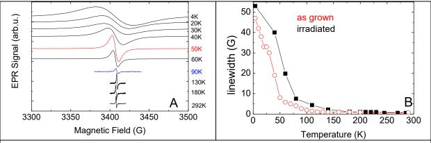
**Figure 4**: temperature dependence of: (A) EPR spectra for B//b , (B)peak-to-peak linewidth  $\Delta B$  of the as grown (red circles) and irradiated (black squares) samples,
