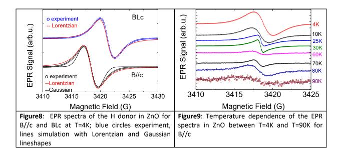
Lorentzian and the peak-to-peak linewidth 2.5G (fig.8). The linewidth for the localized donors in ZnO is much smaller than in the case of Si in  $\beta$ -Ga<sub>2</sub>O<sub>3</sub> due to the small abundance of nuclei with non-zero
