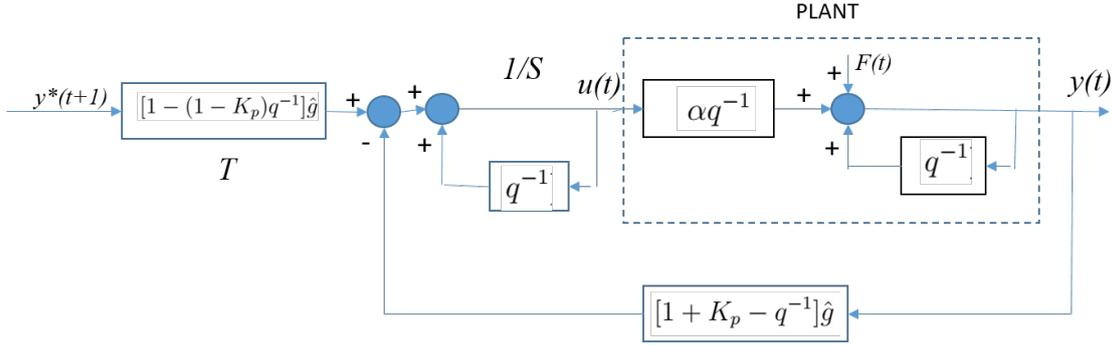
Figure 2: Model Free Control Diagram - R-S-T form.
