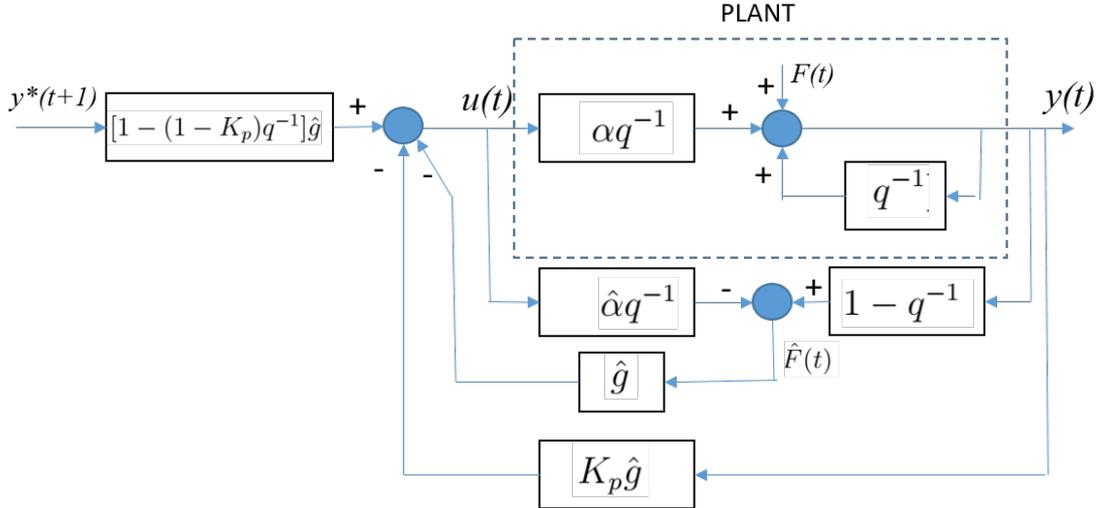
Figure 1: Model Free Control Diagram
