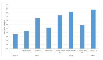
Fig. 9: Execution time with multiple combinations of unrecoverable error in the different middleware check points in the application.
