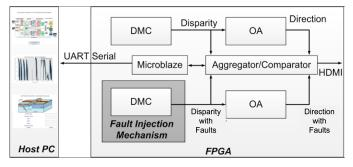
Fig. 3: Experimental Platform - System block diagram
