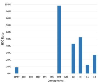
Fig. 5: SDC rate for different components using Obstacle Avoidance Algorithm
