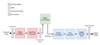
Fig. 8: Pipeline during execution.
