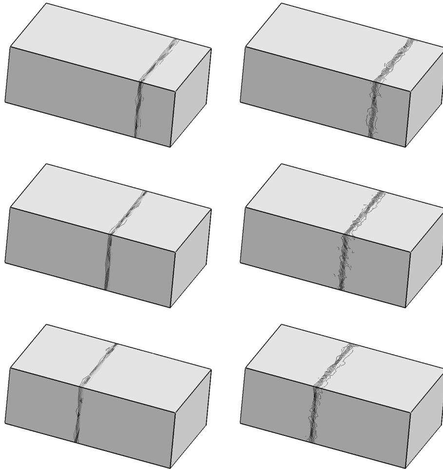
**Figure 11: Density contours after 20 (top), 40 (middle) and 60 (bottom) refinements. The problem has  $\mathcal{O}(150,000)$  degrees of freedom for the anisotropic case (left) and  $\mathcal{O}(450,000)$  degrees of freedom for the non-conforming case (right).**
