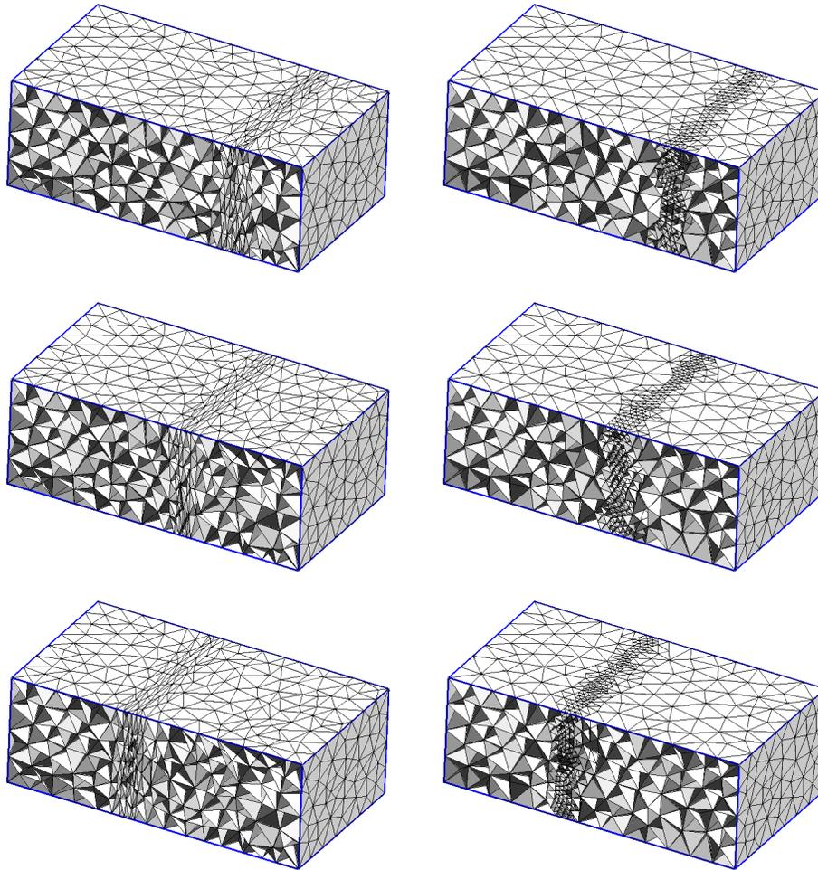
**Figure 12: Meshes after 20 (top), 40 (middle) and 60 (bottom) anisotropic (left) and non-conforming(right) refinements. The triangular faces classified on the front model face have been hidden in order to see interior mesh faces.**
