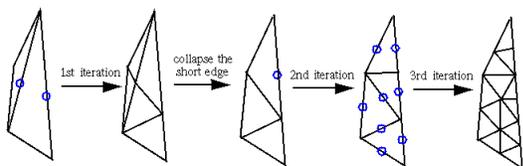
**Figure 5: 2D example of the refinement algorithm.**
