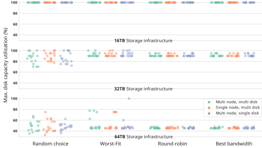
Fig. 5. Maximum disk capacity utilisation (% of capacity), for 16TB, 32TB and 64TB platforms with split strategy and 200G threshold. The 1N1D layout has been removed.
