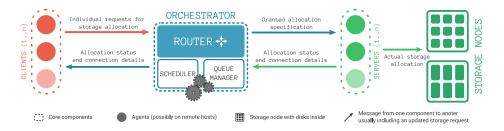
Fig. 2. StorAlloc core scheduling components
