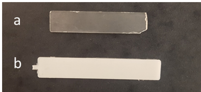
Figure 2. DMA samples of an injection moulded a) neat PLLA, b) PLLA + 1wt% Stear-C4 at 110°C for 75secs
