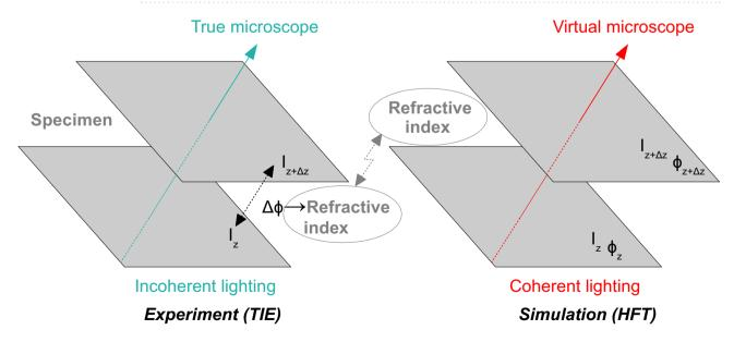
**Figure 5.** Left: experiment with a microscope using incoherent lighting. Right: image simulation using coherent lighting.
