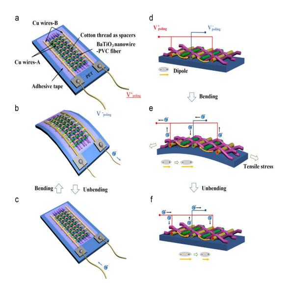
**Figure 9.** Representations of the operating mechanism of the flexible fabric nanogenerator (FNG). (a) FNG structure, (b) Mechanical deformation (Bending) of FNG along the direction of piezoelectric fibres, (c) Unbending of FNG, (d) The status of FNG after poling process where the dipole aligns alongside the direction of the piezoelectric fibre, (e) Carrier flow due to the generation of piezopotentials on the electrodes under the mechanical bending, and (f) under the
