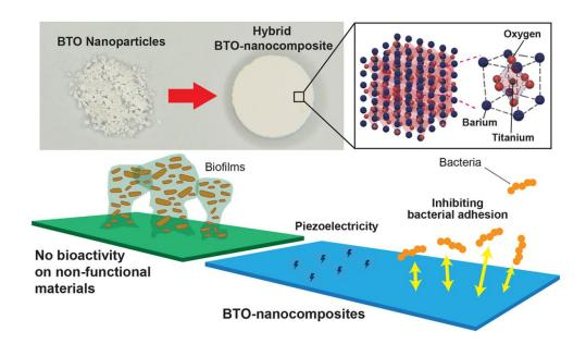
**Figure 11.** Schematic illustration of a bimodal BaTiO<sub>3</sub> nanocomposite platform with antibiofilm and self-powering functionalities Reproduced with permission. <sup>[266]</sup> Copyright 2021, American Chemical Society.
