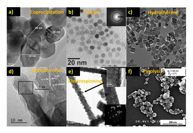
**Figure 5.** Different morphologies and sizes of BaTiO<sub>3</sub> obtained *via* different synthesis' routes: a), c), d), e) and f) Reproduced from publications <sup>[171]</sup>, <sup>[157]</sup>, <sup>[154]</sup>, <sup>[170]</sup>, <sup>[168]</sup> with permission from Elsevier; b) Reproduced with permission. <sup>[89]</sup> Copyright 2001, American Chemical Society.
