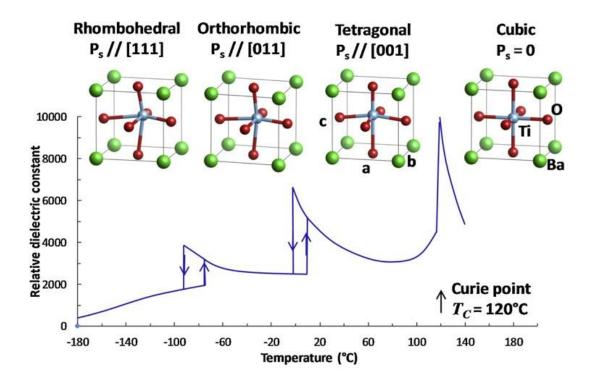
**Figure 3** Evolution of crystal structure and relative dielectric constant as a function of temperature in BaTiO<sub>3</sub> single crystal. Reproduced with permission. <sup>[65]</sup> Copyright 2020, Elsevier.
