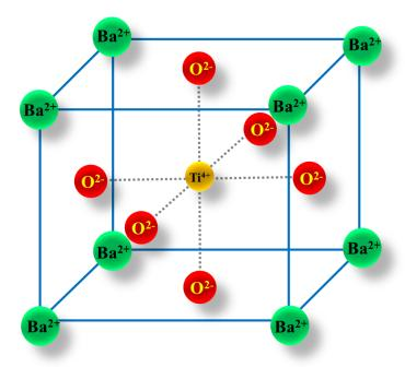
Figure 2. Crystal structure of cubic BaTiO<sub>3</sub> phase
