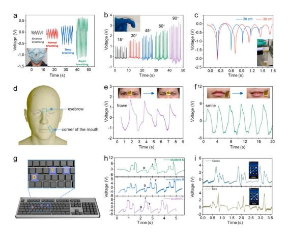
**Figure 10**. Sensing operation of PMNP textile bioelectronics: (a) Real-time output voltage pattern, (b) dynamic output voltage waveforms of finger bending at different angles, (c) dynamic output pattern for free-falling table tennis ball with various falling heights, and (d) schematic model of PMNP textile bioelectronics for active facial expression identification. Real-time output patterns in response to frown (e) and smile (g). Digital images of PMNP
