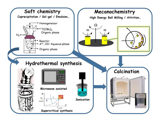
**Figure 4.** Schematic representation of different synthesis routes for the production of BaTiO<sub>3</sub> NPs
