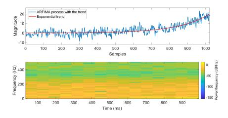
Figure 5: Time representation of an ARFIMA process evolving around its additive exponential trend and its spectrogram
