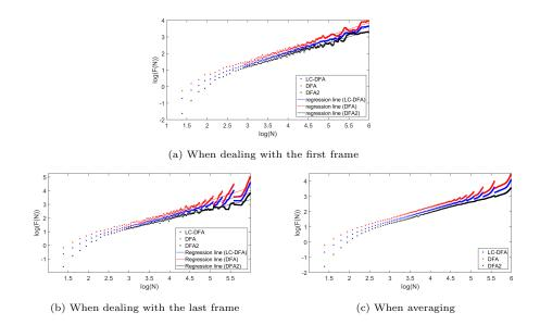
Figure 11: Estimation of the LRD with the DFA, the  $2^{nd}\text{-}\mathrm{order}$  DFA and the LC-DFA with  $\mu=0.4$
