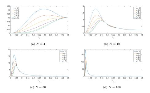
Figure 8: Frequency responses of the LC-DFA with orders 1 and 2 for different values of the weight, for N = 4, N = 10, N = 30 and N = 100
