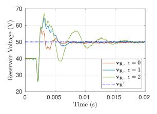
Fig. 8. Experimental measurements of the startup of the converter on the nominal set-point for different values of  $\Omega = \epsilon I d_3$ . Only  $v_R$  is shown, but the same behaviour is observed on the other outputs
