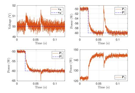
Fig. 6. Experimental measurements of the PFC in closed-loop with control (22). Reservoir voltage and power in each line with their references
