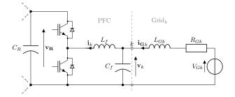
Fig. 2. Detail of the k-th branch of the PFC (left) and the Thevenin grid model as seen by this terminal (right)
