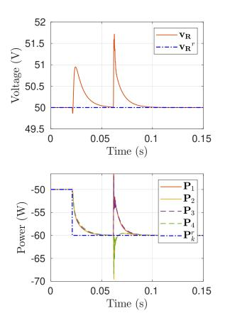
Fig. 9. Simulation of the PFC model (3) for m = 5, in closed-loop with control (22). Reservoir voltage and power in the m - 1 first lines with their references
