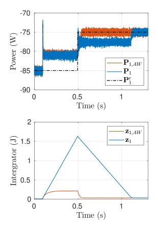
Fig. 7. Experimental measurements illustrating the efficiency of the dead-zone function method to prevent an integral wind-up when the setpoint is unreachable. Power on the first line with its reference (top) and corresponding integrator (bottom)
