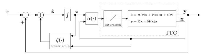
Fig. 3. Proposed control structure for the PFC
