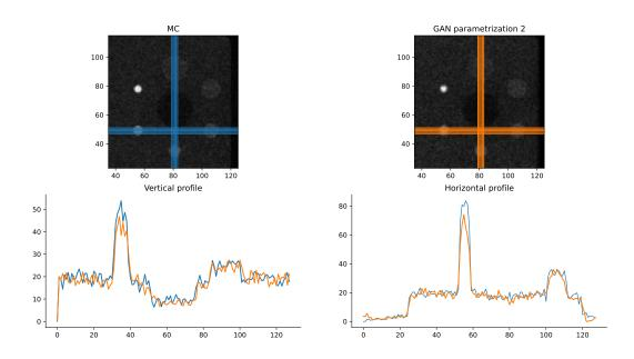
Figure 10: Top panels: slice of the spatial distribution of ideal positions of emission from the second reference phase-space file of experiment 2 (left panel) and from the condGAN-generated phase-space with parametrization 2 (right panel). The horizontal and vertical lines are used for the profiles. Bottom panels : vertical (left panel) and horizontal (right panel) profiles extracted from the top left image (blue) and the top right image (orange). Relative activity recovery is shown in table 6.
