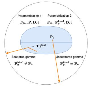
Figure 2: Scheme of the phantom (in blue), the phase-space surface surrounding the phantom and the phase-space parametrization. Gamma sources within the phantom are represented by the initial energy and position of emission ( $E_0$ ,  $P_0$ ). The 8 parameters of parametrizations 1 and 2 are shown. The "ideal" position of emission  $P_0^{ideal}$  is obtained via equation 1.
