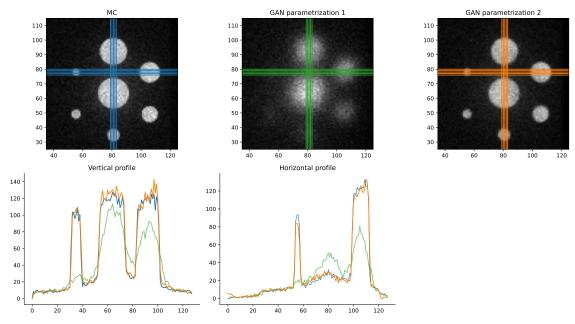
Figure 7: Top panels: slice of the spatial distributions of ideal positions of emission from the reference phase-space file of experiment 1 (left panel) and from the condGAN-generated phase-space, with parametrizations 1 and 2 (middle and right panel). The horizontal and vertical lines are used for the profiles. Bottom panels : vertical (left panel) and horizontal (right panel) profiles extracted from the top left image (blue) and the top middle and right image (green and orange).
