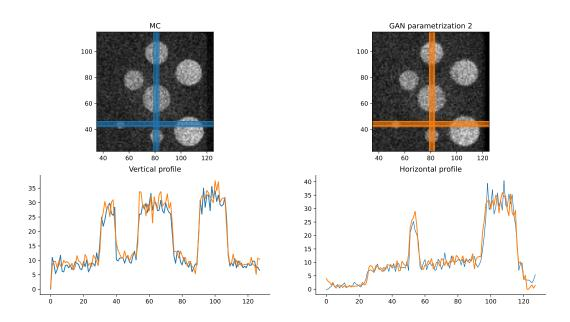
Figure 11: Top panels: slice of the spatial distribution of ideal positions of emission from the third reference phase-space file of experiment 2 (left panel) and from the condGAN-generated phase-space with parametrization 2 (right panel). The horizontal and vertical lines are used for the profiles. Bottom panels : vertical (left panel) and horizontal (right panel) profiles extracted from the top left image (blue) and the top right image (orange). Relative activity recovery is shown in table 7.
