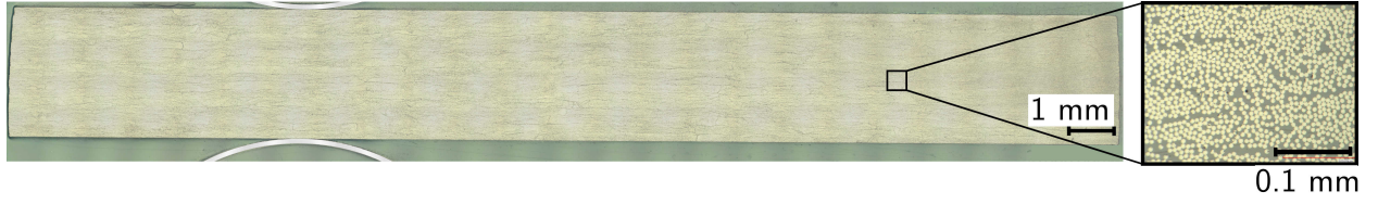
Figure 5: Micrograph of the consolidated samples before deconsolidation tests. The initial porosity content is not measurable.
