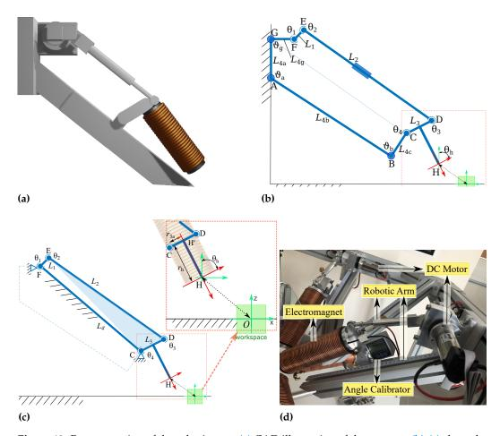
**Figure 12.** Representation of the robotic arm: (a) CAD illustration of the concept, (b)-(c) show the kinematics chain with the four links  $L_1$ - $L_4$  and joints  $\theta_1$ - $\theta_4$ , and (d) represents the realized 1-DOF robotic arm.
