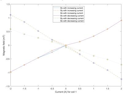
**Figure 24.** Hysteresis curve for the magnetic field at the center of the workspace as a function of current (-2A to 2A) actuating the coil 1. The shape x in the curve denotes the data for increasing current and shape o denotes the data for decreasing current.
