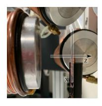
**Figure 23.** The definition of the magnetic directions x, y, z of the sensor TLE493D-W2B6. 23a the front view of magnetic sensor; 23b the side view of magnetic sensor.
