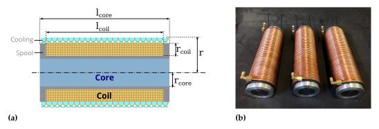
**Figure 9.** (a) illustrates the electromagnet shape, with its core, coil winding and its cooling part. The spool part allows containing the winding and to separate it from the core. (b) presents the implemented electromagnet prototype.
