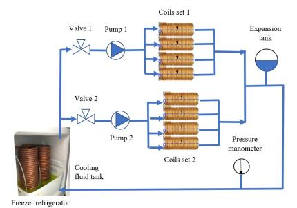
Figure 16. Cooling system for temperature control of electromagnets.
