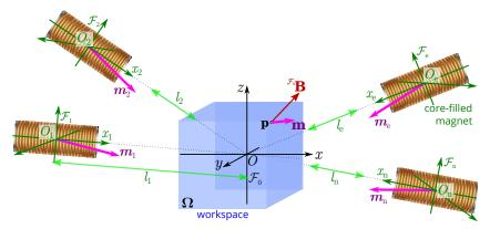
**Figure 4.** Representation of the multipole electromagnets system to induce a magnetic field  $\mathbf{B}(\mathbf{p})$  in the workspace  $\Omega$  (blue square box). The length  $l_e$  denotes the distance between the coil center  $O_e$  to the workspace center O.
