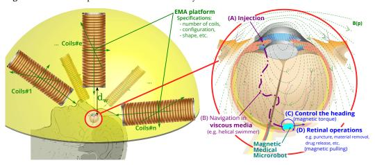
**Figure 2.** Illustration of the ophthalmic microrobotic MIS system: (left) the EMA platform that should respect the geometry of the human head, that is arranged in the yellow hemisphere; (right) the ophthalmic microrobotic MIS procedure where biomedical mirorobot is injected by surgeon and controlled by the EMA setup; the generated magnetic field and gradient induce the magnetic torque and pulling force to the medical microrobot for the different steps of the operations.
