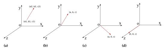
**Figure A2.** Illustration of rotation step along a vector axis. A vector is referred as rotation axis in (a); (b): translate the rotation axis to origin coordinate; (c): rotate the rotation axis to *yoz*-plane; (d): rotate the rotation axis to coincide with *z*-axis. Then the object can be rotated angle  $\theta$  along *z*-axis.
