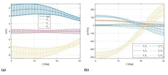
**Figure 17.** The average  $\langle \varphi \rangle$  of the (a) magnetic fields and (b) its magnetic gradients with four moving electromagnets rotating with angle  $\beta \in [0^{\circ}, 45^{\circ}]$ . The error bar shows the standard deviation of the value.
