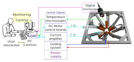
Figure 15. Synoptic of OctoRob platform architecture.
