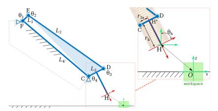
**Figure A1.** Representation of the robotic arm kinematics chain with the four links  $L_1$ - $L_4$  and joints  $\theta_1$ - $\theta_4$ .
