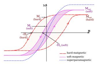
**Figure 5.** Typical hysteresis curve for ferromagnetic materials. The intercepts  $\mathbf{H}_c$  and  $\mathbf{M}_r$  are the intrinsic coercivity and magnetization remanence.
