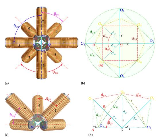
**Figure 6.** Representation of the geometric arrangement of the 3D n=8 electromagnetic coils: (a) top views; (c) side views where three electromagnetic coils are removed to show clearly internal space; (b) and (d) show the geometry between the electromagnets center  $O_e$ . The plain lines depict the in-plane lengths, whereas dashed lines represent the out-of-plane one.
