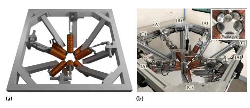
**Figure 13.** OctoRob design. (a) CAD representation of the EMA platform and (b) experimental prototype: (A) 1-DOD mobile robotic arms; (B) optical microscope with a CCD camera; (C) stationary robotic arms.
