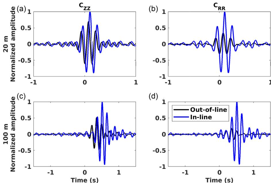
**Figure A2.** Comparison of synthetic  $C_{ZZ}$  and  $C_{RR}$  waveforms between the in-line and out-of-line source cases. The top row is for the 20 m interstation distance sensor pair; the bottom row is for the 100 m interstation distance sensor pair. Each waveform is bandpass filtered between 4.5 and 9 Hz and then normalized by the maximum amplitude of the in-line crosscorrelations so that relative amplitudes are preserved.
