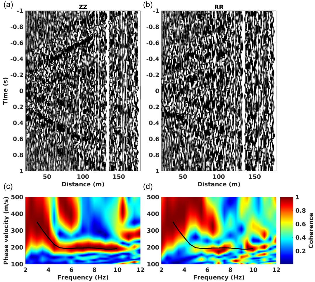
**Figure B1.** The virtual shot gathers of  $C_{ZZ}$  (a) and  $C_{RR}$  (b) after applying a 1 m bin-stack to all crosscorrelations. We apply the phase-shift transform to the sum of causal and acausal parts of the crosscorrelations to generate the dispersion images (c and d). The black lines in the two dispersion images are the smoothed phase velocities from  $C_{ZZ}$ . The waveforms are band-pass filtered between 2 and 12 Hz.
