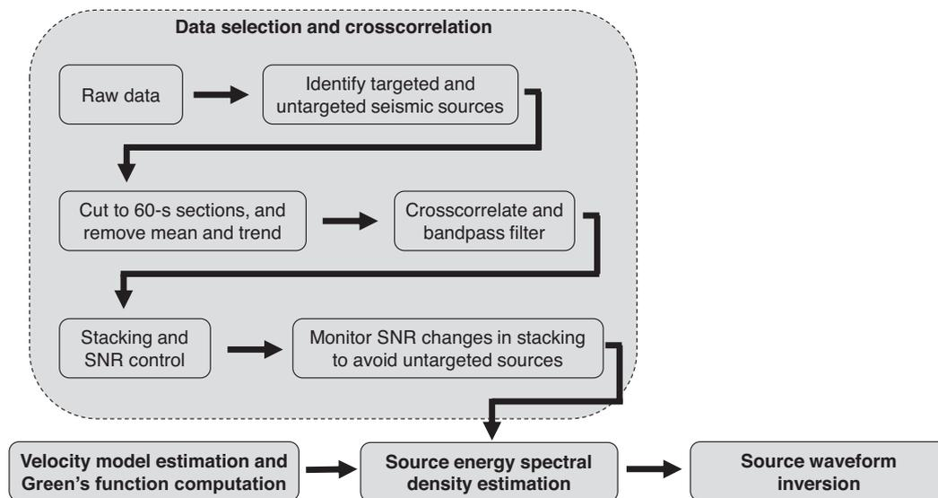
**Figure 2.** The source inversion workflow is divided into four steps: data selection and crosscorrelation (Section 2.1), velocity model estimation and Green's function computation (Section 2.2), source energy spectral density estimation (Section 2.3) and the source waveform inversion (Section 2.4).
