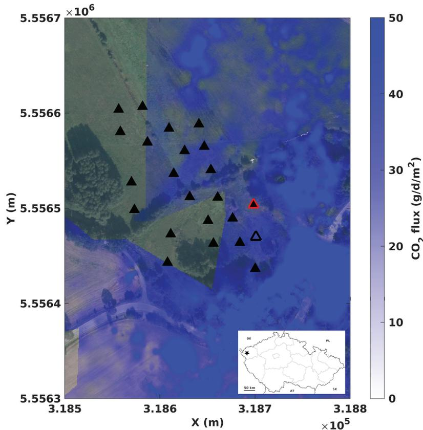
**Figure 1.** A site map of the seismic array and CO<sub>2</sub> gas-flux distributions. Each triangle is a geophone. The empty triangle is the noisy one. The red-edge triangle is the C601 sensor in Fig. 4. The gas-flux data are from Nickschick *et al.* (2015) and were acquired from 2007 to 2013. The star in the inset shows the site location in the Czech Republic. The coordinates are in WGS84/UTM zone 33.
