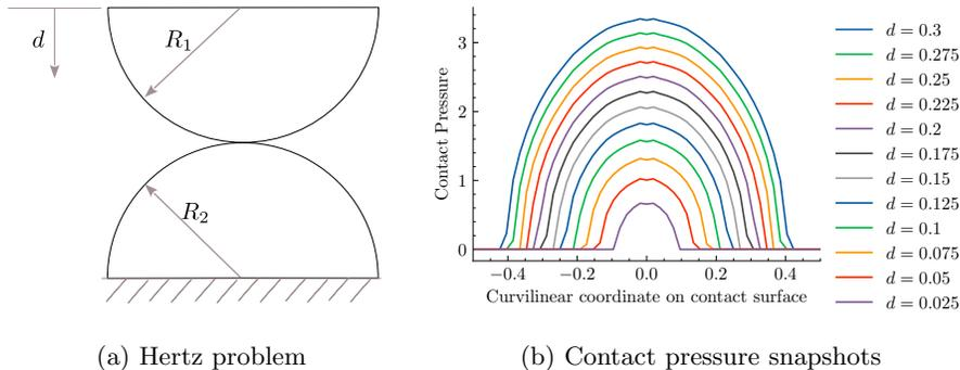
Figure 6: Left: Hertz problem: Two half cylinders loaded against each other. Displacement  $d$ , imposed on the top cylinder, is treated as parameter in the reduced model. Right: Contact pressure snapshots
