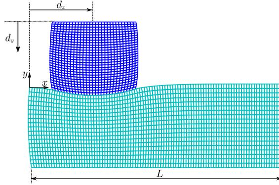
Figure 11: Ironing problem: Iron block is pressed against the flat slab by a displacement  $d_y$  and moved horizontally. The horizontal displacement of the iron block  $d_x \in [0, L]$  is treated as the parameter in the reduced model
