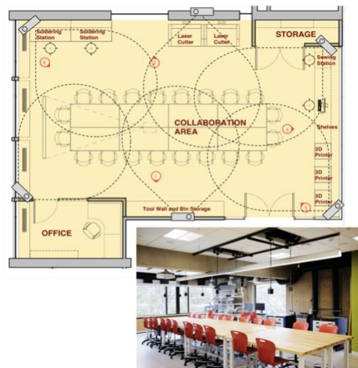
Figure 1. Layout of makerspace with positions and fields of vision of the Kinect sensors (top). Picture of the makerspace (bottom)
