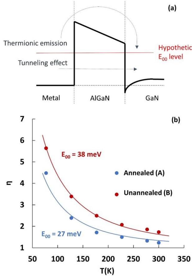
FIGURE 5. Schematic Ni/AlGa<sub>N</sub>/Ga<sub>N</sub> band diagram indicating the preferred electron path according to the  $E_{00}$  level (a). Ideality factor as a function of temperature. Solid lines represent Padovani fits (b).
