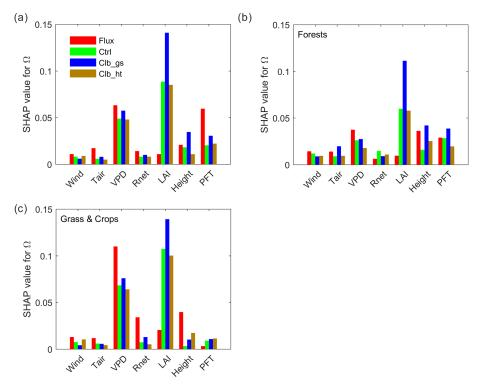
**Figure 4.** Importance of different factors based on absolute SHAP values of  $\Omega$  (the expectance of factor-induced deviation of  $\Omega$  from the averages of all samples). (a) Random forest model built by data from all PFTs. (b) Model using only forest data. (c) Model using only grassland and cropland data.
