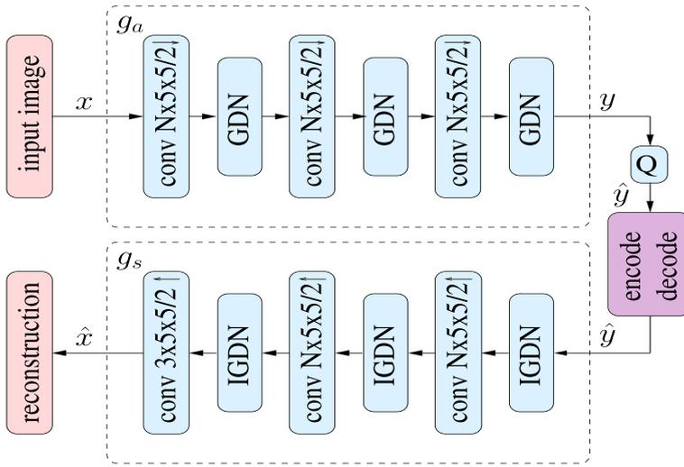
Fig. 1 Block diagram of the baseline end-to-end image compression algorithm [4]
