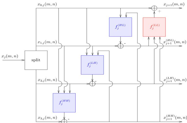
**Fig. 3** Block diagram of the fully connected network based lifting coding scheme [11]
