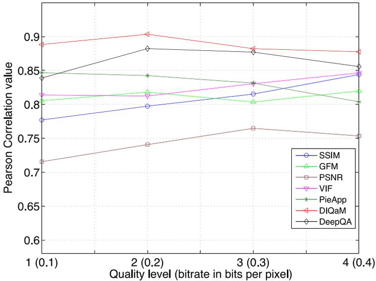
**Fig. 10** PLCC Performance of IQA metrics with respect to the compression quality level
