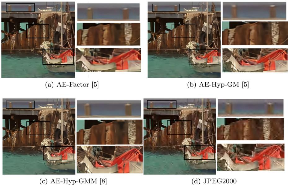
**Fig. 6** Image distortions with JPEG2000 and NN based compression methods (at bitrate of 0.2 bits per pixel)
