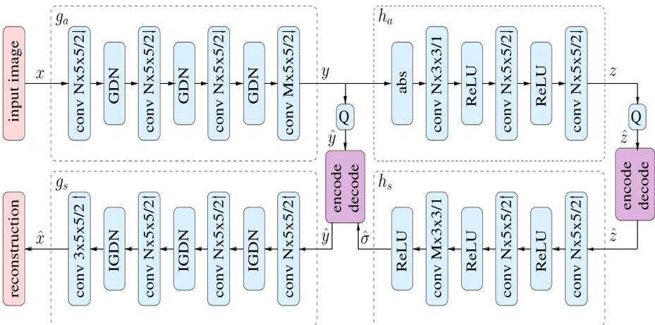
Fig. 2 Block diagram of the end-to-end image compression algorithm with a scale hyperprior [5]
