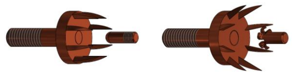
Fig. 6. Sketches of cathode - anode system before explosion (left) and after explosion (right). The cathode-anode system as part of the unit is shown in the sketch, see Figure 4.
