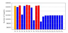
Figure 1: The binary size and the found number of gadgets in  $S_0$  (baseline) and  $S_1 - S_{20}$  (specializations). (mean  $\pm$  std) for binary size -  $S_0$ : (3,096,176  $\pm$  0),  $S_{1-20}$ : (3,020,417  $\pm$  63,641), and for gadgets -  $S_0$ : (106,495  $\pm$  0),  $S_{1-20}$ : (103,414  $\pm$  2,696)
