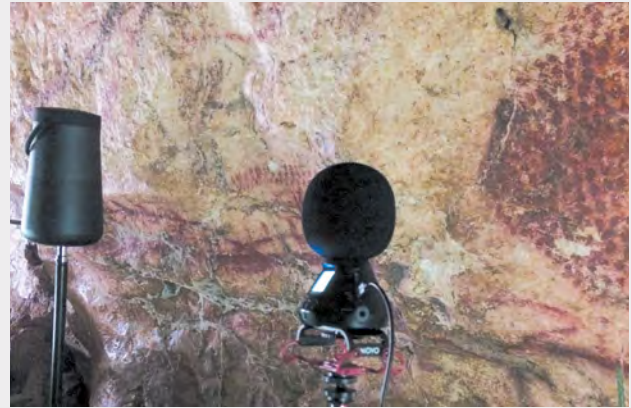
Figure 5. Experimental setup for acoustical impulse-response measurements in the central section of the Marsoulas Cave, adjacent to its iconic, red-dotted bison image (right). A portable omnidirectional loudspeaker and spatial audio recorder were used in this fieldwork conducted by Kolar, Nerness and Valentin in September 2021. Photo by Barbara Nerness.
