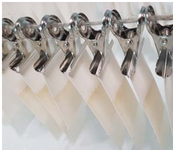
Figure 2: Tidelines formed on the artificially aged samples by dipping their lower end of the paper in water for 1h30 (machine direction is vertical).
