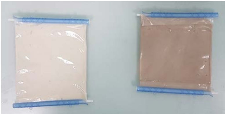
Figure 3: Regenerated cellulose membrane filled with B (left) and S (right) ready to be used.
