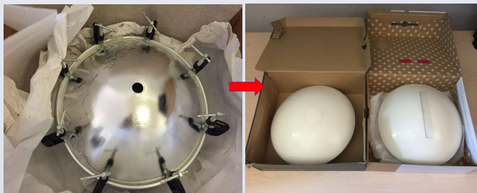
Fig.1. The molding process of a dielectric paraffin lens and the fabricated paraffin wax lenses
